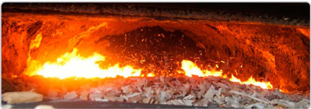
Figure 3: Testing of Wood Chip in Coal Fired Rotary Drum Drier
