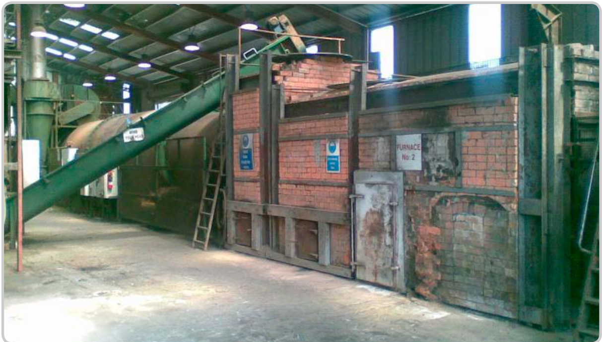
Figure 1: Direct Coal Fired Rotary Drum Drier
